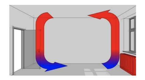
An interchange flow is established between hot air going up and cold air going down.
